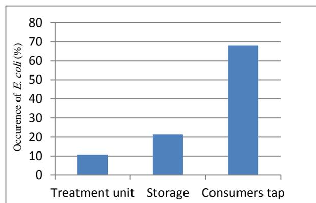
**Figure. 3:** Occurrence of *Escherichia coli* in drinking water in treatment unit and distribution system.
