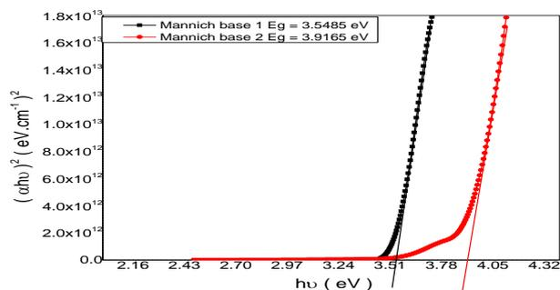
**Figure (3)** the energy band gap spectrum of compound 1 and 2
