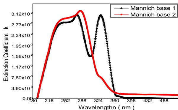
**Figure (4)** the Extinction Coefficient spectrum of compound 1and 2
