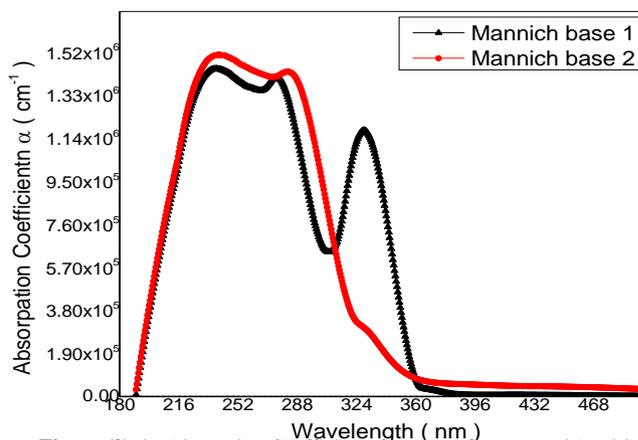
Figure (2) the Absorption Coefficient spectrum of compound 1 and 2
